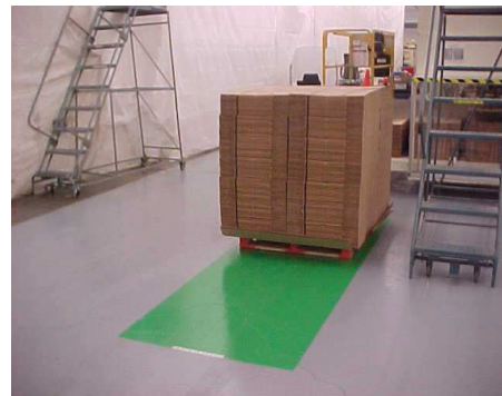
After: Organized and color coded space which also acts as a kanban
